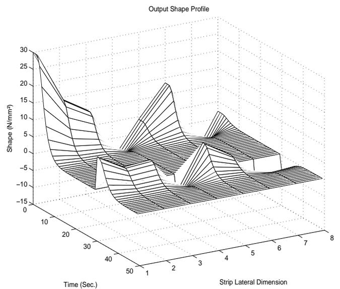
Fig. 5. Shape profile evolution for high order PFC
