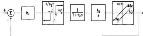
Fig. 2. Block diagram of the actuator subsystem
