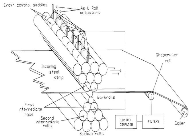
Fig. 1. The Sendzimir cold rolling mill
