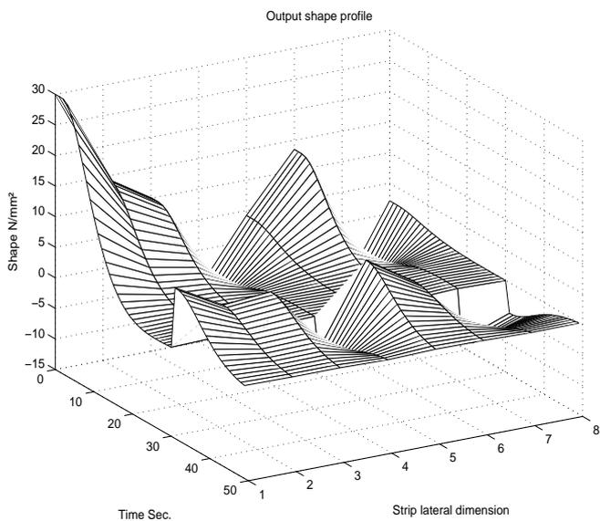
Fig. 7. Shape profile evolution for PID controller
